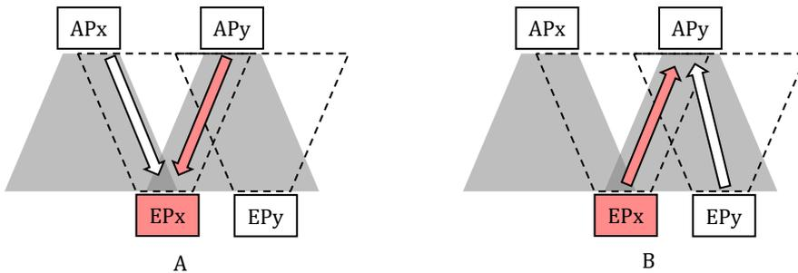
**Figure 2 Interference for downlink transmission (A) and uplink transmission (B)**
