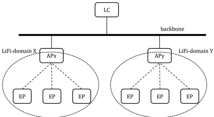
**Figure 3 LiFi network architecture**
