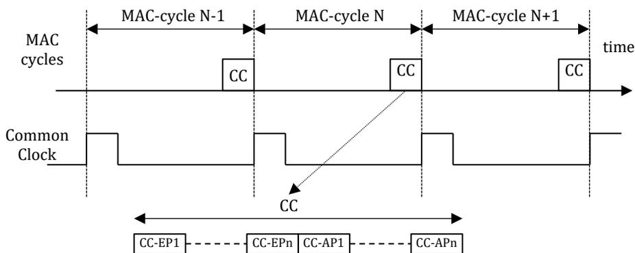
**Figure 4 MAC cycle alignment to common clock and CC**
