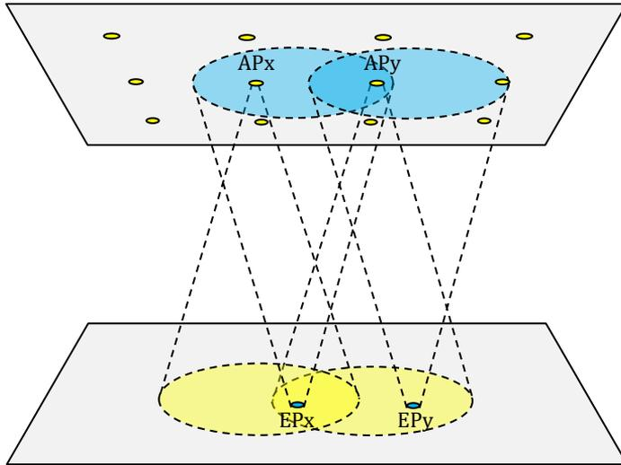
**Figure 1 Situation with LiFi Access Points (AP) in ceiling and LiFi End Points (EP)**
