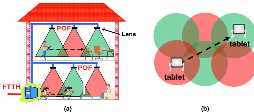
**Fig. 1:** An in-home network employing luminaire-free LiFi transmission systems using POF and lens (a) and wireless cells (b) with an example of user's movement crossing several wireless cells.
