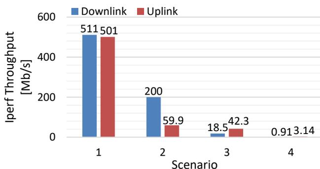
**Fig. 3: Throughput measured using IPerf software for the four link conditions using G.hn for phoneline profile: Scenario 1: Low correlated channel. Scenario 2: User OFEs are closely placed and are positioned in the middle of the coverage area. Scenario 3: User OFEs are closely placed and are positioned in front of one of the OFEs of the ceiling node. Scenario 4: One of the OFEs of the user node is blocked.**
