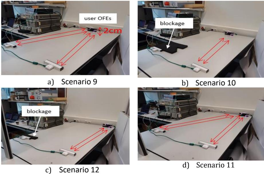
**Fig. 6: Test arrangement where the user OFEs are placed together to model practical use cases.**
