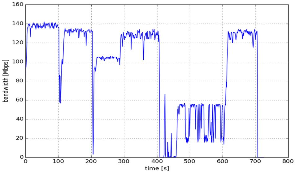
**Fig. 9: Link performance when moving user-side OFEs, blocking and un-blocking one of the ceiling-side OFEs.**
