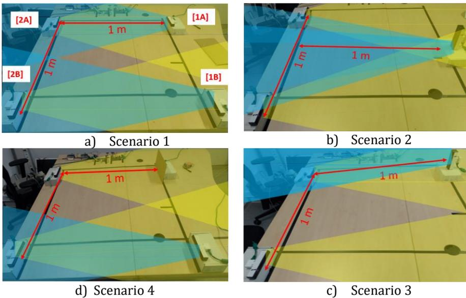
**Fig. 2: Illustration of the four different link conditions investigated with G.hn for phoneline profile.**
