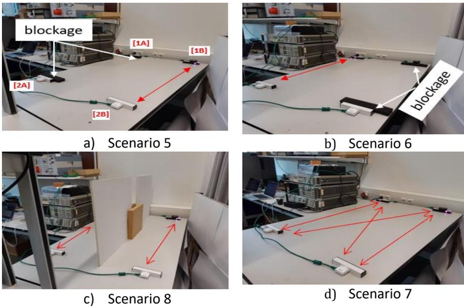
**Fig. 4: Test setup arrangements to evaluate link performance of G.hn for powerline profile in MIMO LiFi when the user side OFEs are spaced by 60 cm.**
