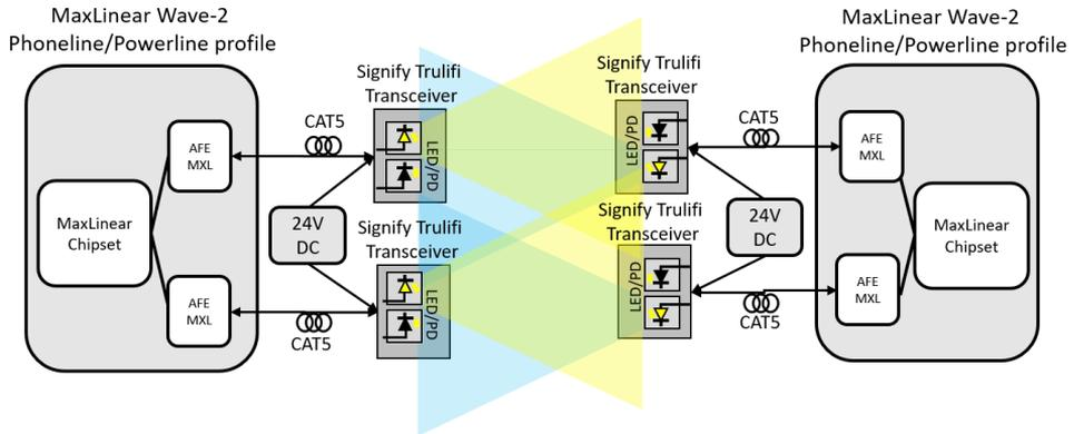
**Fig. 1: G.vlc in MIMO LiFi with phonline or powerline profiles.**
