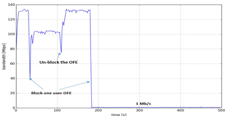
**Fig. 8:** Link performance when changing channel characteristics by blocking one of the user-side OFEs, before software upgrade to improve adaptation.
