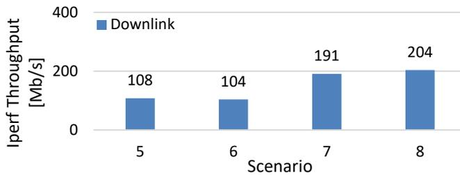
**Fig. 5: Throughput measured using IPerf software for link conditions 5-8 using G.hn for powerline profile.**
